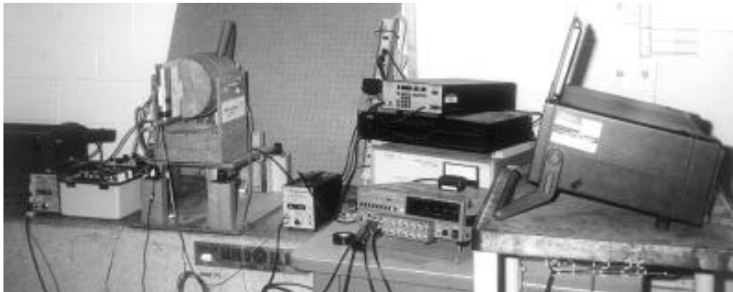
Figure 9. Picture of system set-up for ISO Standard 10819 tests.
