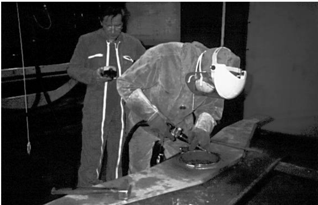
Figure 1. Measurement of vibration emitted by a rotary file being used to fettle a component.
